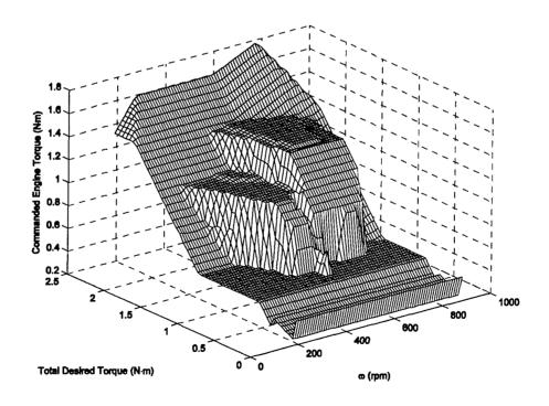
Figure 6-15: Engine Torque Control Surface, Two-Stroke, Three-Input Algorithm, Charge-Depletion, SOC=25%
