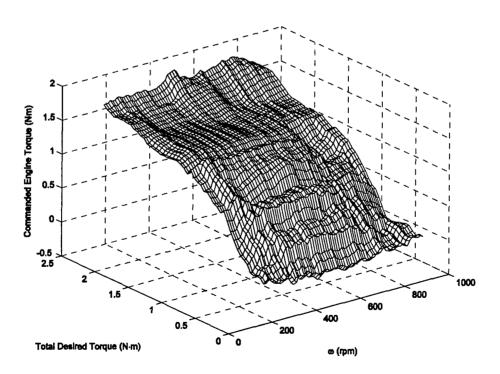
Figure 6-35: CMAC Approximation (L=9) for Engine Torque Control Surface (see Figure 6-17), Four-Stroke, Three-Input Controller, Charge-Depletion, SOC=25%
