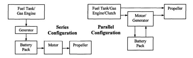
Figure 1-1: Series and Parallel Hybrid-Electric Configurations
