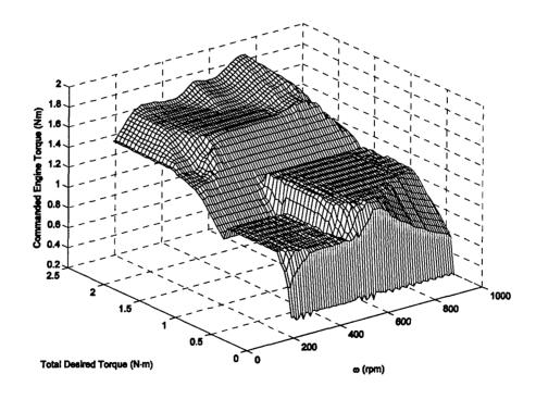
Figure 6-25: CMAC Approximation (L=3) for Engine Torque Control Surface (see Figure 6-11), Two-Stroke, Three-Input Controller, Charge-Sustaining, SOC=25%
