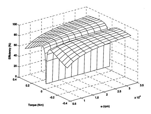
Figure 6-4: Motor Efficiency Map
