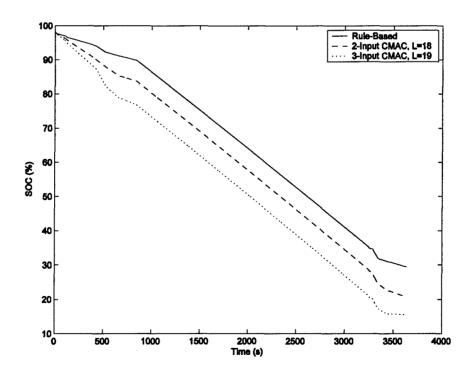
Figure 6-47: Battery SOC, One-Hour Mission, Four-Stroke, HEUAV Configuration, Rule-Based and CMAC Controllers, Charge-Depletion
