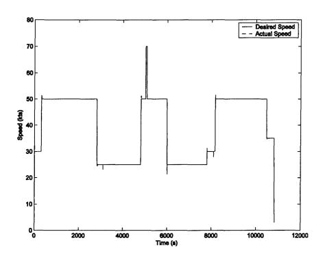
Figure 6-56: Desired and Actual UAV Speed, Three-Hour Mission, Four-Stroke, HEUAV Configuration, Three-Input CMAC Controller (L=14), Charge-Sustaining
