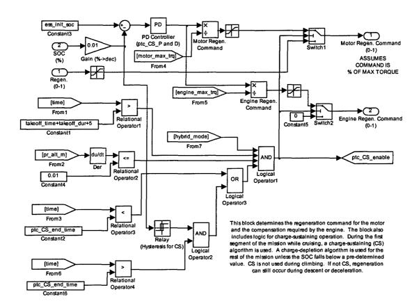
Figure 4-10: Regeneration/Charge-Sustaining Logic Block
