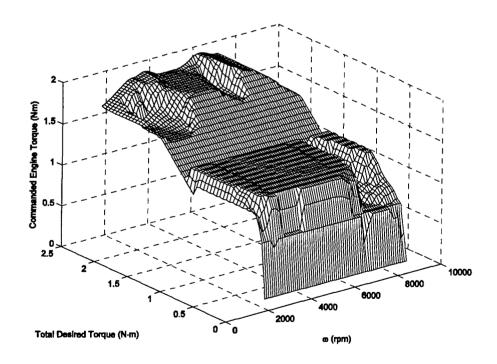
Figure 6-13: Engine Torque Control Surface, Four-Stroke, Three-Input Algorithm, Charge-Sustaining, SOC=25%
