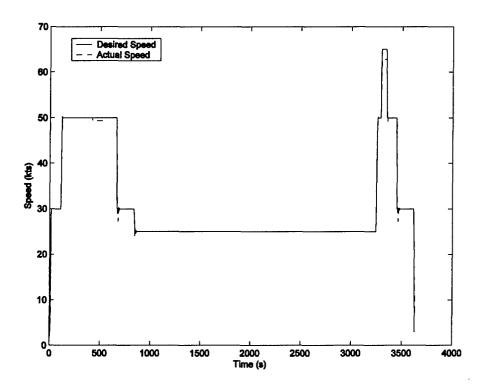
Figure 6-44: Desired and Actual UAV Speed, One-Hour Mission, Four-Stroke, Original Configuration
