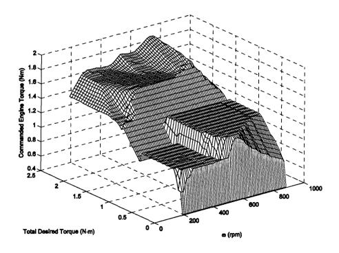
Figure 6-11: Engine Torque Control Surface, Two-Stroke, Three-Input Algorithm, Charge-Sustaining, SOC=25%
