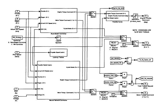
Figure 4-9: Propulsion System Controller Model
