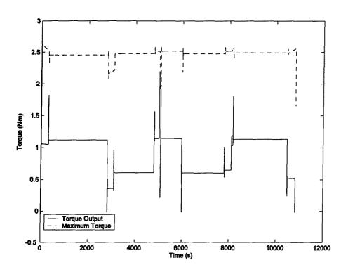
Figure 6-59: Engine Torque, Three-Hour Mission, Four-Stroke, Original Configuration
