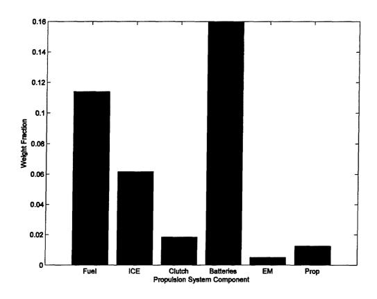
Figure 5-5: Weight Fractions for the HEUAV Propulsion System
