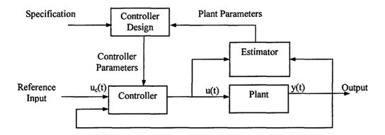
Figure 2-3: Block Diagram of an Indirect Adaptive Controller
