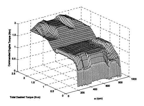
Figure 6-29: CMAC Approximation (L=3) for Engine Torque Control Surface (see Figure 6-13), Four-Stroke, Three-Input Controller, Charge-Sustaining, SOC=25%
