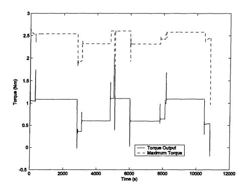
Figure 6-51: Engine Torque, Three-Hour Mission, Two-Stroke, Original Configuration
