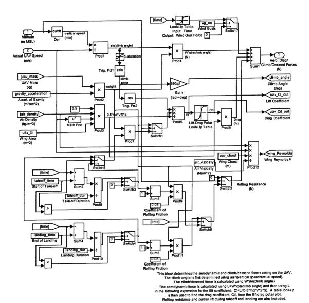
Figure 4-13: UAV Forces Model
