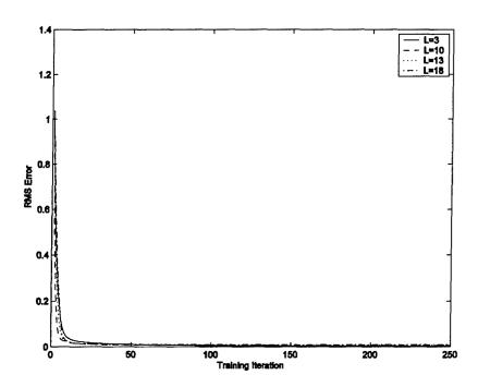
Figure 6-21: RMS Error, Two-Stroke, Two-Input Controller
