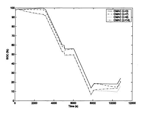
Figure 6-65: Battery SOC, Three-Hour Mission, Four-Stroke, HEUAV Configuration, Three-Input CMAC Controllers, Charge-Sustaining
