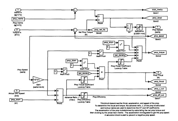
Figure 4-11: Propeller Model
