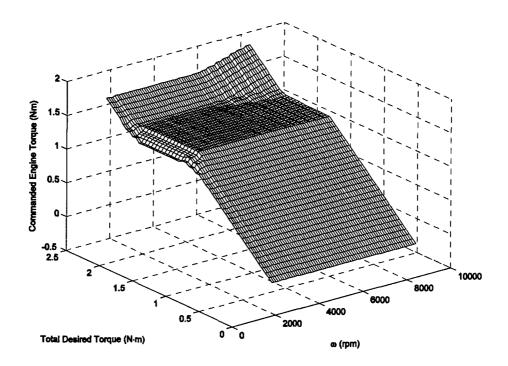
Figure 6-22: CMAC Approximation (L=18) for Engine Torque Control Surface (see Figure 6-8), Four-Stroke, Two-Input Controller
