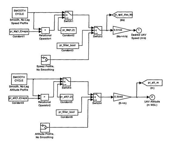
This block determines the desired speed and altitude of the UAV. If pr\_filter\_bool is true, a centered-in-time average of the profile is required. This is useful to smooth out jumps in the flight profile.
