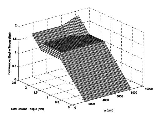
Figure 6-8: Engine Torque Control Surface, Four-Stroke, Two-Input Algorithm
