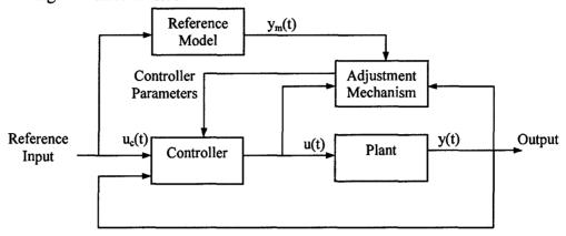
Figure 2-2: Block Diagram of a Direct Adaptive Controller
