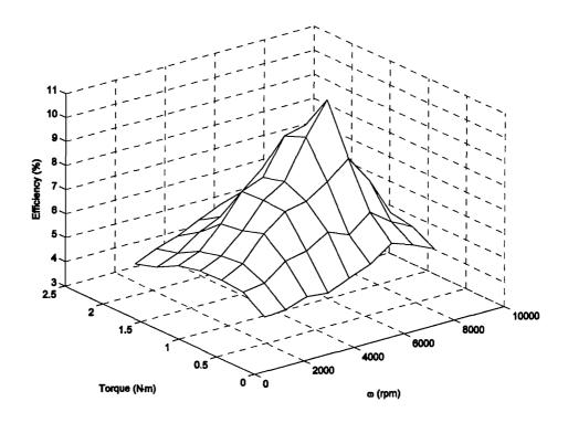
Figure 6-2: Two-Stroke Engine Efficiency Map
