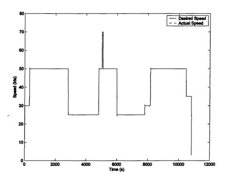
Figure 6-64: Desired and Actual UAV Speed, Three-Hour Mission, Four-Stroke, HEUAV Configuration, Three-Input CMAC Controller (L=14), Charge-Sustaining
