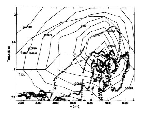
Figure 6-41: Engine Operating Points, One-Hour Mission, Two-Stroke, HEUAV Configuration, Three-Input CMAC Controller (L=19), Charge-Depletion
