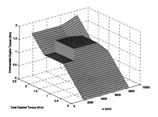
Figure 6-7: Engine Torque Control Surface, Two-Stroke, Two-Input Algorithm
