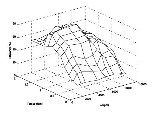
Figure 6-3: Four-Stroke Engine Efficiency Map
