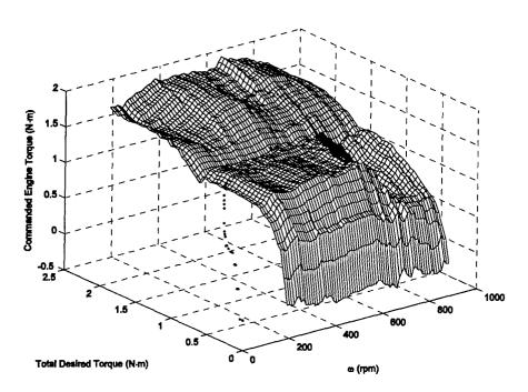
Figure 6-69: Engine Torque Control Surface and Operating Points, Cruise Mission Segment with Wind Turbulence, Four-Stroke, HEUAV Configuration, CMAC Controller (L=14), Charge-Sustaining
