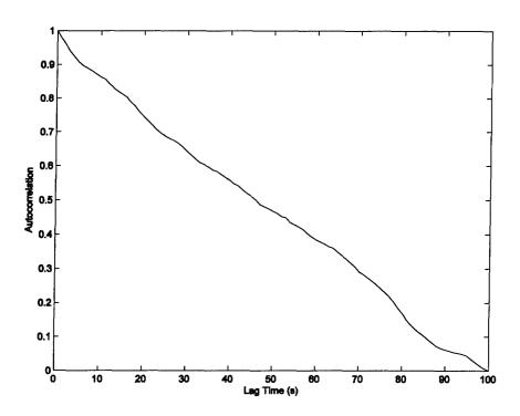
Figure 6-66: Autocorrelation of Sample Wind Turbulence
