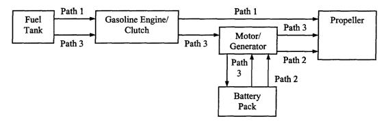
Figure 6-1: Energy Paths Available in the Hybrid-Electric System
