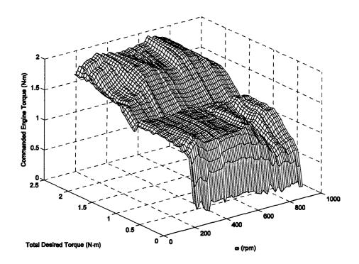
Figure 6-31: CMAC Approximation (L=14) for Engine Torque Control Surface (see Figure 6-13), Four-Stroke, Three-Input Controller, Charge-Sustaining, SOC=25%
