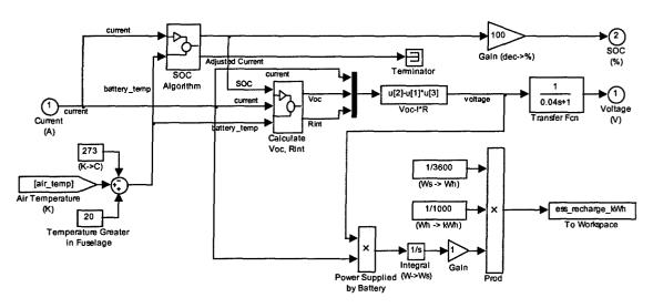
This block models the energy storage system as a voltage source in series with an internal resistance.
