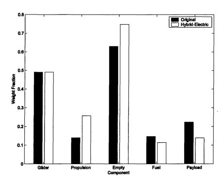
Figure 5-4: Weight Fractions, Normalized to UAV Weight
