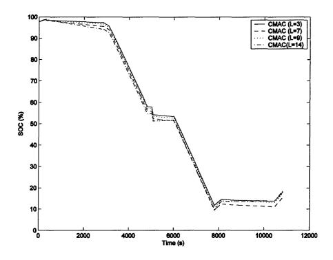
Figure 6-57: Battery SOC, Three-Hour Mission, Two-Stroke, HEUAV Configuration, Three-Input CMAC Controllers, Charge-Sustaining
